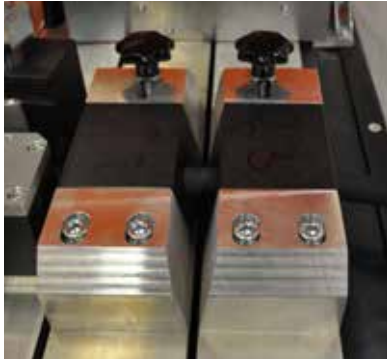
Prebend system for best cut result and to ensure long lifetime of the blade
